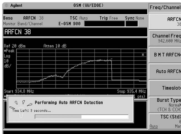
Figure 3. Automatic carrier frequency and band selection to simplify measurements.
